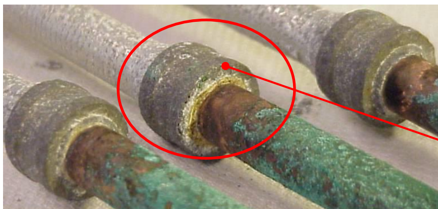
Chem Lab Control # 4144, Lokrings, CCT Test, Vertical in cabinet, aluminum toward top, 4362 hours
