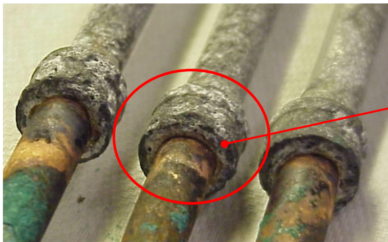
Chem Lab Control # 4144, Lokrings, CCT Test, Horizontal in cabinet, 4362 hours
