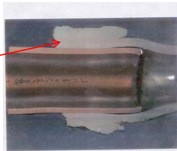
Horizontal Copper Tube/Aluminum Tube Lokring Sample After Cyclic Corrosion Test.
